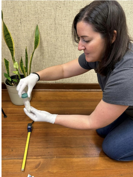
In this picture Katie Baldwin, Supervisor of Regulated Facilities and Housing, is collecting a dust wipe of a floor in a home. She places the wipe in a clean tube which is then sent to the lab to be analyzed for lead content in the floor dust. The result should be less than 10 \mu\text{g}/\text{ft}^2 .
